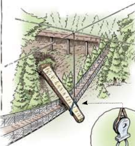
Fig 4:- 17 tons of downward force means a lot of upward cable force. Quick removal would create a "slingshot effect" propelling everything onboard skyward.
